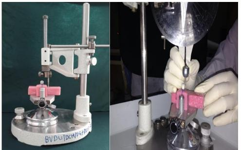
Fig 2: Surveyor used to acheive parallelism.
